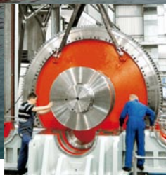
Twin Marine Gear Units „Dual-Fuel / Electric Propulsion“ Typ: NDSH-4000 Power: 2 x 14.8 MW Speed: 720/90,6 rpm
