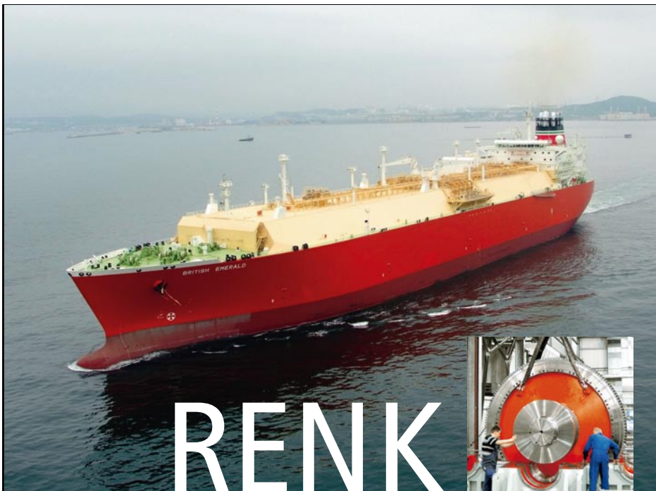
Twin Marine Gear Units „Dual-Fuel / Electric Propulsion“ Typ: NDSH-4000 Power: 2 x 14.8 MW Speed: 720/90,6 rpm
