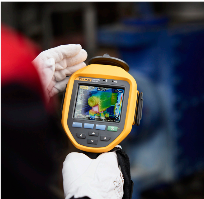
Thermal imaging is one of the methods of identifying gas leakage, which can lead to reduced efficiency and reliability in a compressor
