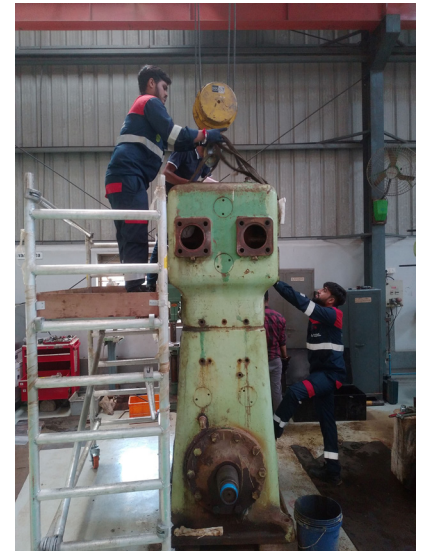
30-year-old Laby® compressor being dismantled
