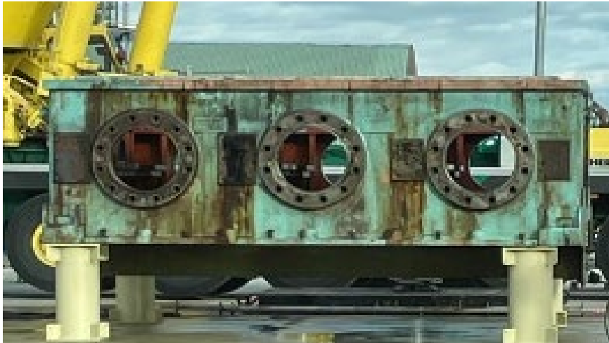
Crankcase of Nuovo Pignone hyper compressor
