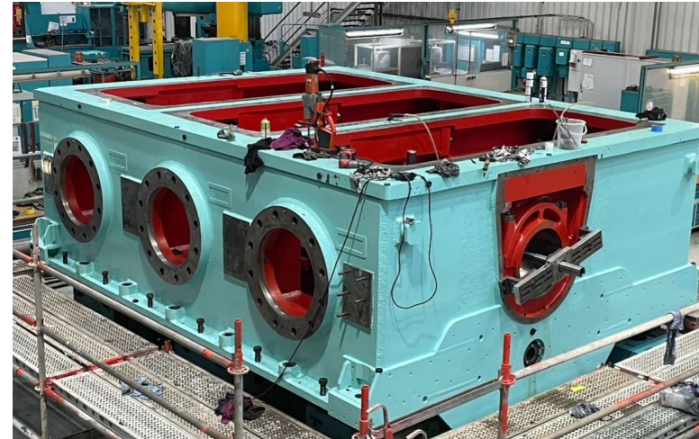
Repaired crankcase at Burckhardt Compression workshop
