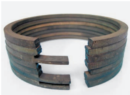
Fig. 2 Step-cut piston rings made of a brittle polymer blend and exhibiting fracture of the overlapping joints
