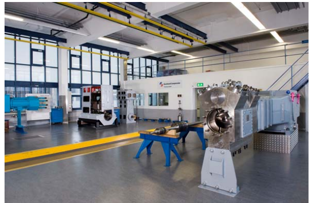
The modernized Training Center showing from left to right a cylinder of the Hyper Compressor, the Laby ® Compressor and on the right side the Process Gas Compressor
