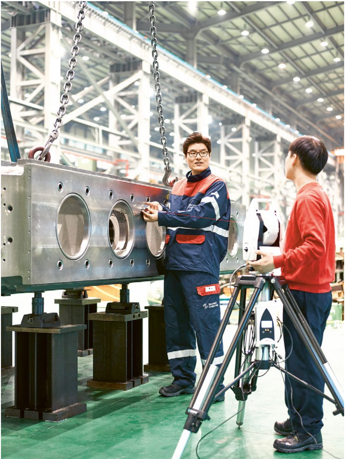
The Tracker's laser beam detects the reflector on the workpiece to be measured itself. This allows measurements to be taken quickly and with extremely high precision.
