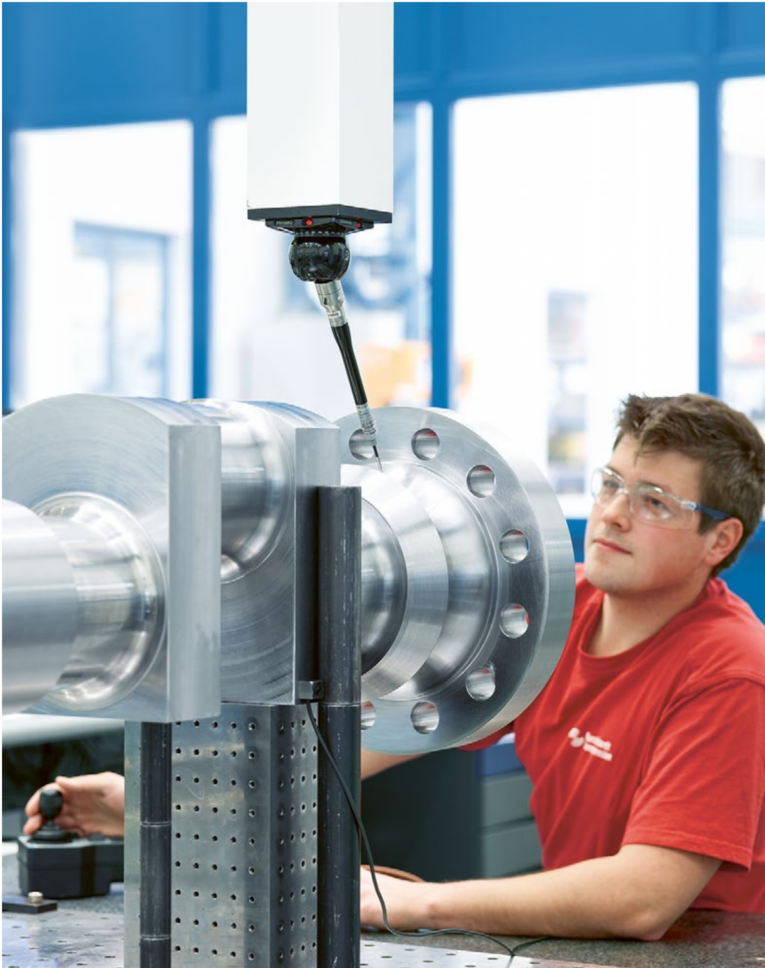
The laser measuring room is kept cooled to a constant 19 °C (66 °F) to ensure precise results.
