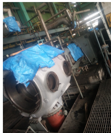
Revamped compressor cylinder during assembly
