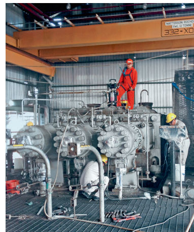
One of the three F6 hyper/secondary compressors
