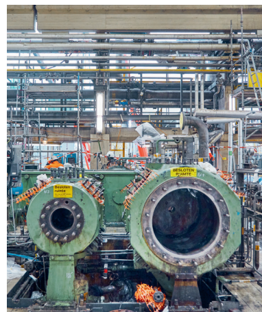
Compressor before revamp with indications of leakage.
