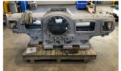
Frame after sandblasting
