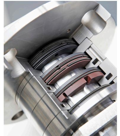
Piston and packing rings were upgraded to Persisto® 850, a material specially developed for dry-running applications.
