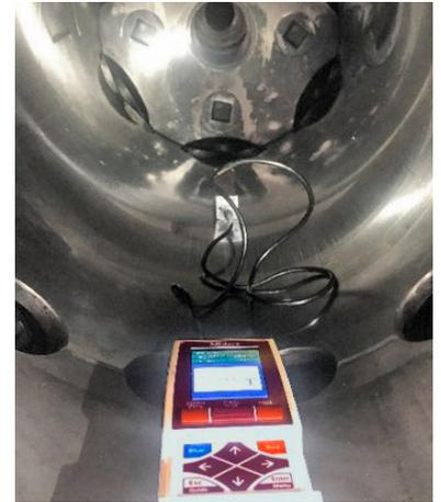
Proper surfaces roughness is critical. Thorough analyses showed that the surface of the cylinder liner was too smooth.
