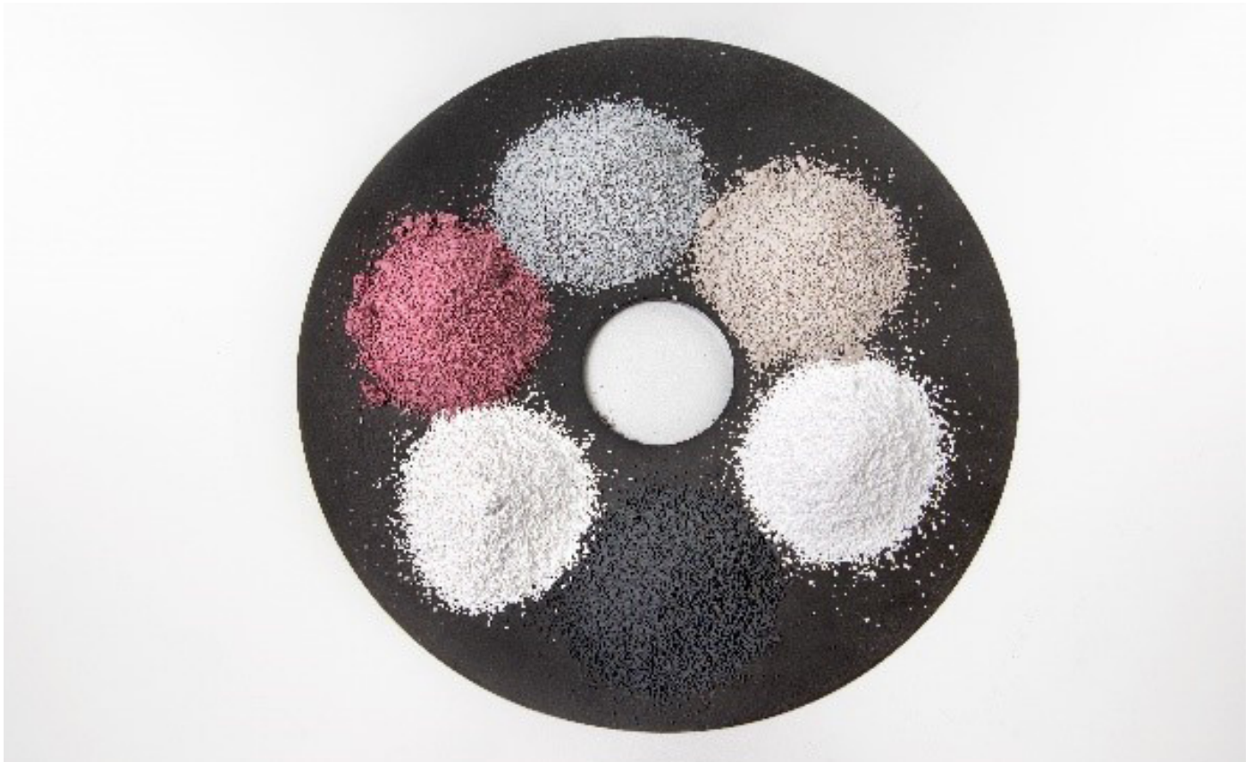
Image 1: Burckhardt Compression develops its own Persisto® material specifically suited for reciprocating compressors
